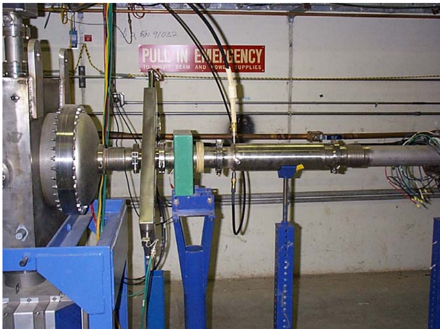
Figure 6. The downstream end of the Chopper. A small wide-aperture vertical pulsed dipole will be placed just after the Chopper, followed by a horizontal pulsed dipole. A new arrangement of the wire scanner, Pierson transformer and Griffin monitor will provide the needed space.
